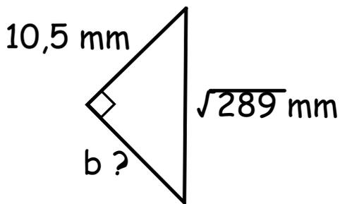
$$\begin{aligned} h^2 &= a^2 + b^2 \\ (\sqrt{289})^2 &= 10,5^2 + b^2 \\ 289 &= 110,25 + b^2 \\ 289 - 110,25 &= 110,25 - 110,25 + b^2 \\ 178,75 &= b^2 \\ \sqrt{178,75} &= \sqrt{b^2} \\ 13,4 \text{ mm} &\approx b \end{aligned}$$
